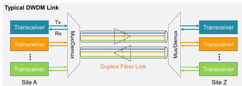
Figure 4. Typical DWDM link which may or may not be amplified.
