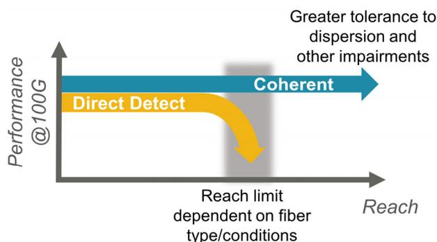
*Figure 8. Direct-detect solutions hit a reach limit at a certain distance while the coherent solution will continue to operate beyond this reach limit.*
