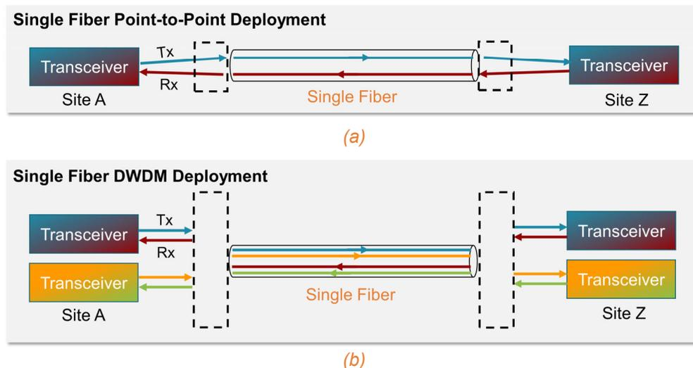
Figure 5. Optical transmission in a service provider edge/access network over (a) a single fiber BiDi link and (b) a DWDM single fiber BiDi link—in both cases, the transmit wavelength is different from receive wavelength for each data transmission stream. The optical implementation to combine signals into a single fiber depends on the link requirements.
