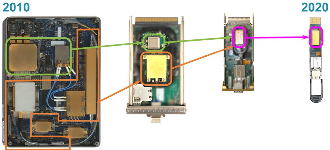
Figure 10. Evolution of coherent module size over time.
