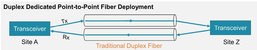
Figure 2. Typical dedicated point-to-point fiber link.
