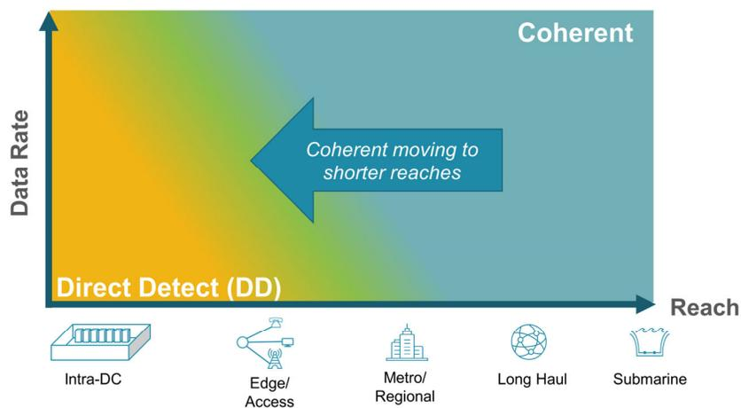
Figure 6. Coherent solutions are evolving towards shorter reaches.
