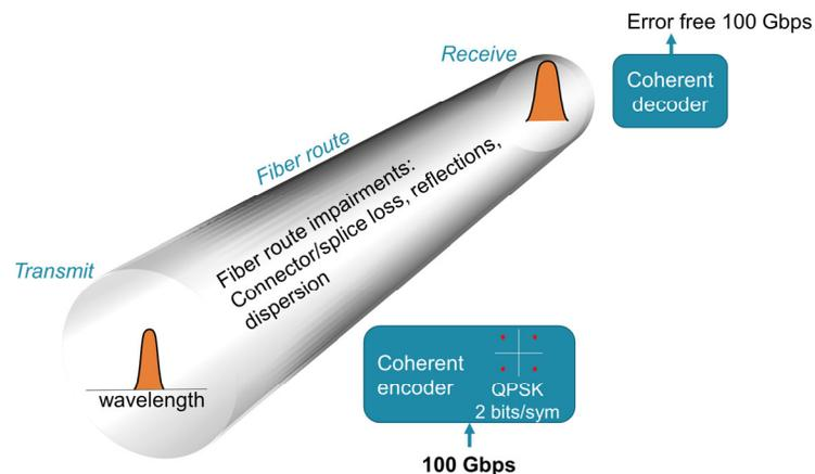
Figure 7. Error-free coherent transmission of 100Gbps QPSK modulation example, tolerant to multiple impairments (only one transmission direction shown).
